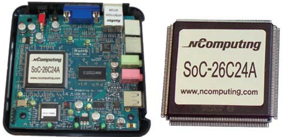
The NComputing System-on-Chip (SoC) is at the heart of each access device
